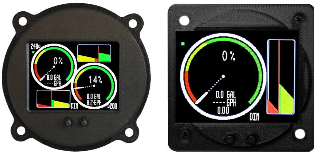
2 1/4" Dual Resistive and Single Capacitive, both showing graphing over time.
