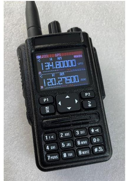
*AirLite Pro™ demonstrating dual channel simultaneous aircraft reception*
