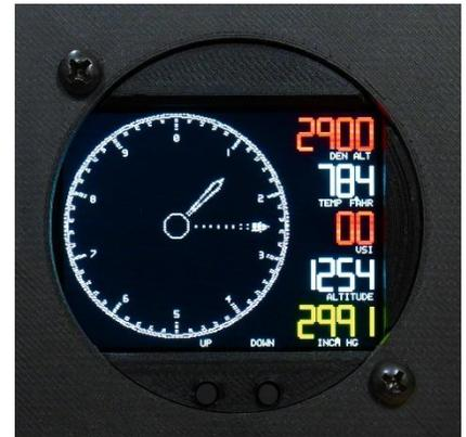
*Gen2 Altimeter showing traditional 2 needle face along with digital VSI, temperature and Density Altitude*
